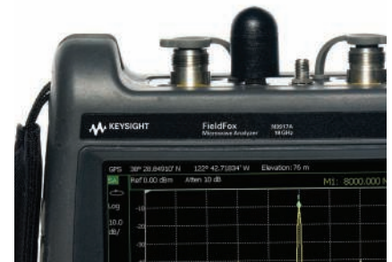
Use the built-in GPS to obtain geo-location data
